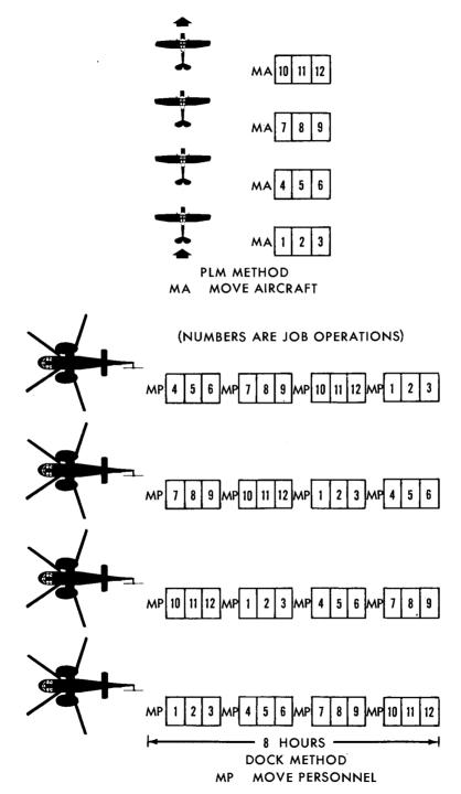
Figure 11-1. Comparison of dock and production line methods.
