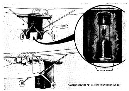
Figure 11-3. Preheating with a plumber's pot.
